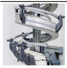
The spiral elevator is a compact and high throughput solution for up or down elevation. It ensures a continuous product flow while the elevation is as simple and reliable as a normal straight conveyor. The spiral-shape is the key to its unique compact construction that saves valuable floor space. The application range is wide, from the handling of individual parcels or totes to handling of packed items such as shrink-wrapped bottle packs or cartons.
