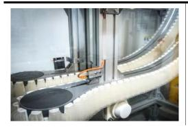
A wedge conveyor uses two conveyor tracks facing each other to provide fast and gentle transport both horizontally and vertically. Wedge conveyors can be connected in series, if proper timing of the product flow is taken into account.
