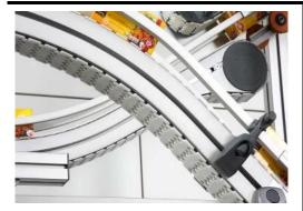
The incline elevator conveyor is designed for single or multiple lane elevation. It provides gentle handling of sensitive product and is easy to adjust for different products sizes. This conveyor can be complemented with friction top chain to achieve steeper inclines.
