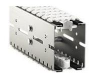
Standard conveyor widths range from 70 mm up to 300 mm, for product widths up to 500 mm. Suited for items with a weight up to 30 kg. Stainless steel conveyor systems are designed for demanding production environments where contamination or chemical exposure is a potential risk. For this reason they are an ideal solution for the food processing, pharmaceutical and personal care industries where hygiene and regular wash downs are critical.
