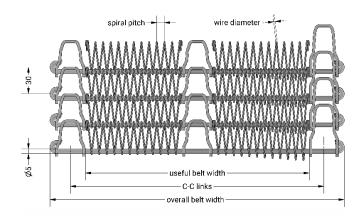
**Space saver –** Constructed with a double row of non collapsing links on the inner edge. When turning, the outside edge expands while the inner edge remains extended. Products do not get "wrinkled" or damaged as the belt does not collapse
