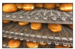
FlexCAM provide a range of wire mesh belts to suit new and existing conveyors. These are usually found in food processing applications such as Cooling, Freezing, Proofing, Steam cooking, Baking and the like.
